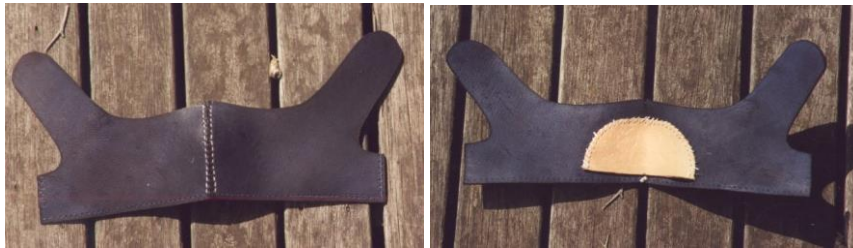
Front and back views of the quarters, showing the stitching (not visible from the inside) and the counter.
