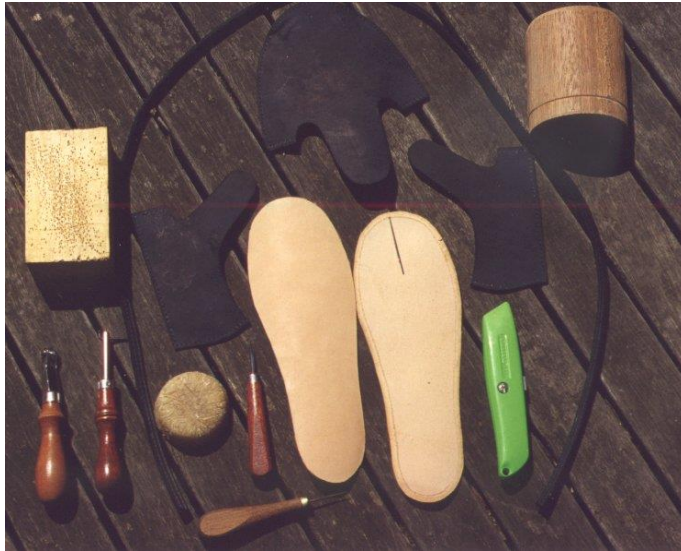
All tools and parts required to make a latchet shoe.
